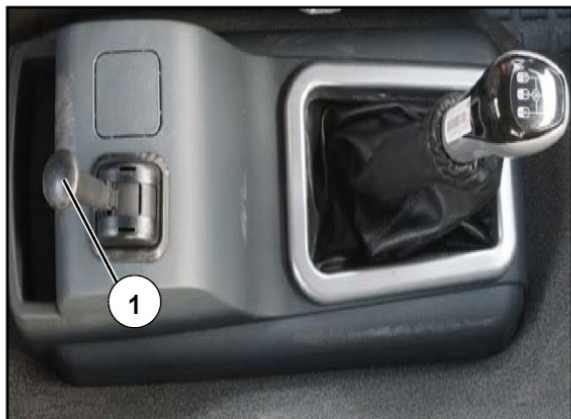
The driving spring energy storage brake chamber – parking brake release
